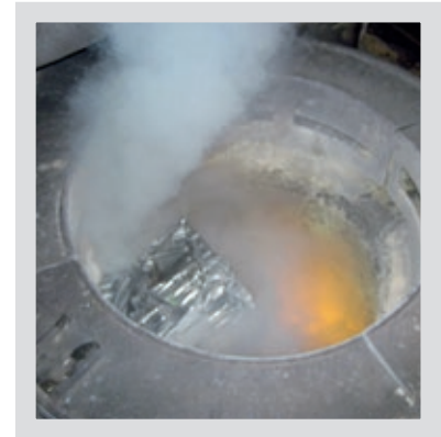
A CIF for brass melting lined with silica dry product
